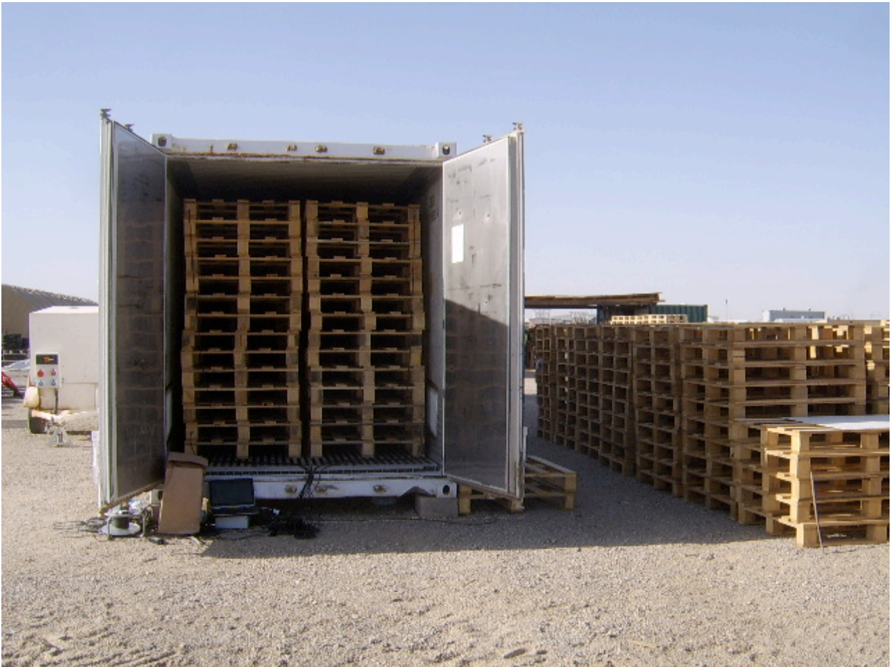
Up to 250 pallets like these can be heat treated for ISPM15 in a Thermokil 40' container conversion
